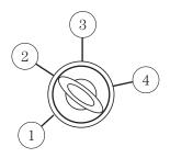
4. Start— cranks the engine. Release the key as soon as the engine starts.
